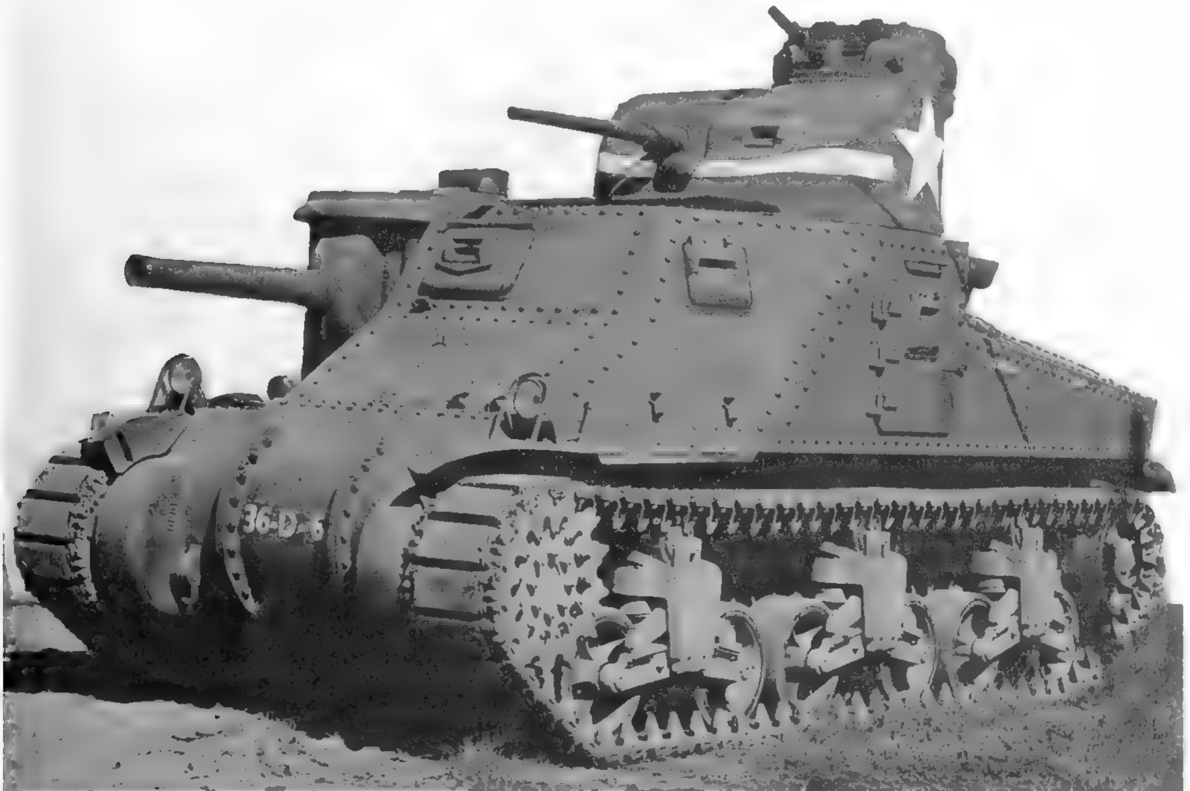
The M3 was designed as a stopgap. While unusual looking and of questionable combat effectiveness, it was very effective as a test bed for the chassis that would be the basis of the later Sherman. The many rivets that held the M3 together are visible in this photograph. (Photo courtesy of the Patton Museum)
